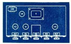
Fig. 1. Chassis layout.
