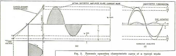
output tube used to illustrate the cause of harmonic distortion.
