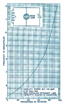
Fig. 3. Absorption wavemeter calibration.
