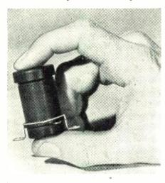
device with the normally-open contacts rated at 10 amperes direct current. These contacts will make or break 30 amperes at altitudes up to 40,000 feet.
