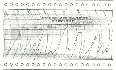
Fig. 6. Typical record sheet from the Lie Detector machine, showing response curve.
