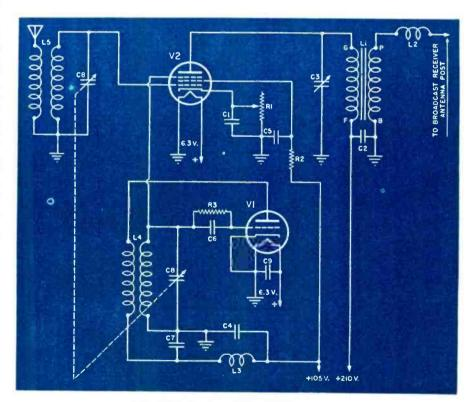
Schematic diagram of the R-F Converter.
