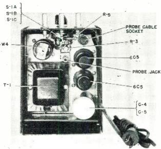
Fig. 3. Rear view showing a.c. probe inserted in its jack.
