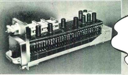
Unique and revolutionary methods have been developed by Harvey engineers for the production and assembly of communication receivers ... which separate the circuits of the receivers into basic circuit-elements by the use of standardized R. F., I. F. and Audio cells that are complete self-contained circuits. Mass production is achieved by this method with important improvements in sensitivity and selectivity.
