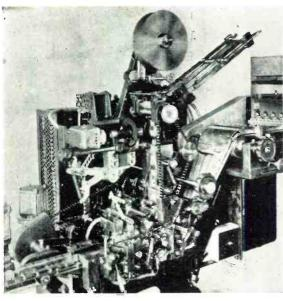
Cellophane wrapping machine using photoelectric relay to synchronize cutting and printing.
