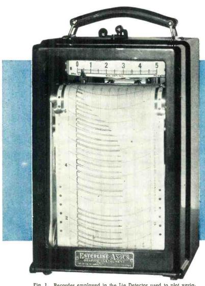
Fig. 1. Recorder employed in the Lie Detector used to plot variations in skin resistance and heart amplitude simultaneously.
